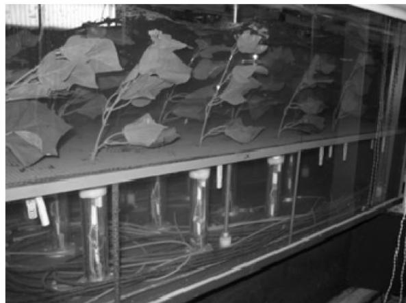
**Fig. 1: Setup of DFS test section and artificial poplars under flow action.**
